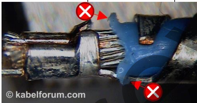
Error: Uncleanly cut, frayed insulation
